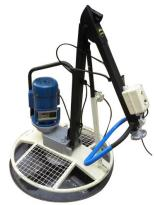
The **Concrete Power Trowel** with electric motor is a high efficiency, light weight machine for floating & toweling concrete surface. the machine can be operated at two speeds 115 and 57 R.P.M. to obtain the desired output. This machine is provided with two types of finishing tools. A disc for floating and a set of four bleds for toweling. to obtain fine finish the blade angle should be control.
